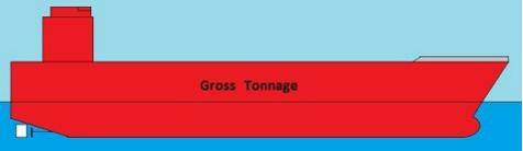
Gross Tonnage is a measure of the ships total **<u>interior volume</u>** and is calculated by multiplying the interior volume "V" of the ship in cubic meters by a variable known as "K" (which varies depending on the ships overall volume).
