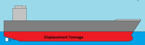
Displacement tonnage is nothing more than the total weight of the volume of water a ship "displaces" when it is sitting in the water.
