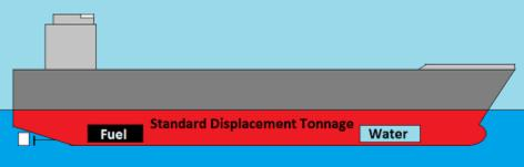
Standard displacement tonnage = "displacement tonnage" – ( the weight of any fuel and potable water carried on board the ship )
