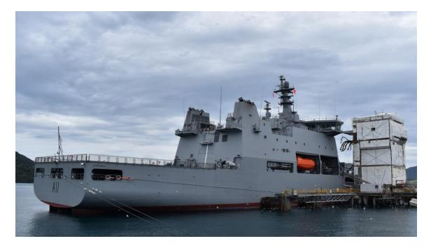
The Royal NZ Navy's new Replenishment Tanker HMNZS *Aotearoa* A11 delivered by Hyundai this year on her first call to Marsden Point Refinery to uplift 10000 tonne of diesel fuel . Ship is ice classed to enable her to carry out Antarctic fuel deliveries to McMurdo Station. Photo : Bryan Shankland ©
