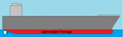
Lightweight tonnage is best described as the weight of the ship when it was built in the shipyard including all framing, machinery, decking, etc.
