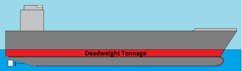
Deadweight tonnage is the weight (in tons) of all the cargo, fuel, dry provisions, supplies, etc. carried on board the ship.
